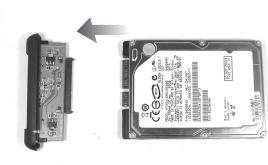
4-2 Insert the hard drive caddy back into the NexStar CX housing as the picture
